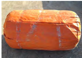
Before switchover: Nylon-covered polystyrene foam floats
