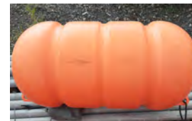
Post-switchover example: PE-coated polystyrene foam floats
