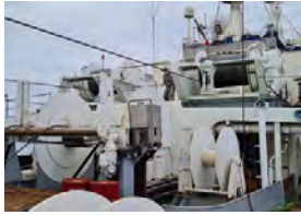
Automatic Trawl Winch of EMDEPES
