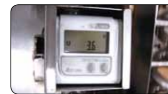
An instantaneous flow meter that shows how many liters of water per minute are used
